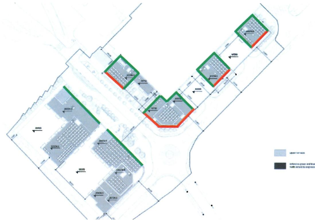
**Figure 7** Facades Requiring Upgraded Sound Insulation
